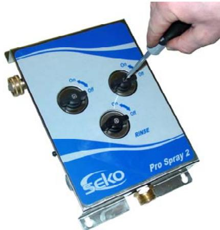
◀2 Remove valve knobs and set tools aside.
