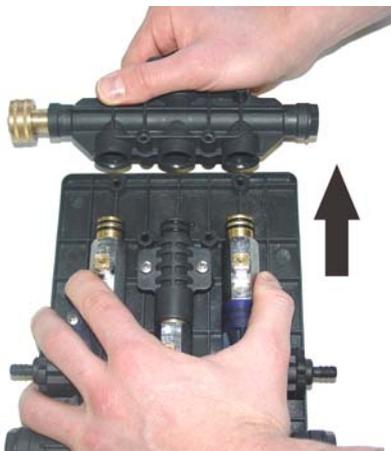
◀1 Take apart the upper manifold, rock the ball valve back and forth to make the manifold easier to disassemble
