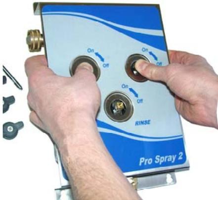
◀3 Place thumbs on valve stem and lift from the underside of the facing
